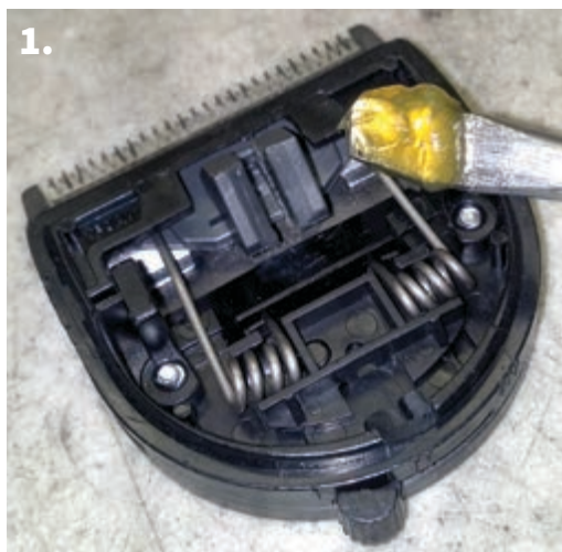
CLOCKWISE FROM LEFT: 1.) 5-N-1 Blade before greasing. 2.) 5-N-1 after greasing. 3.) Oiling the rear of blade. 4.) Oiling the front of blade.
